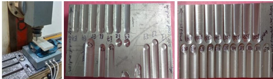
FIGURE 3.1: Universal Vertical Milling Machine & work-pieces
