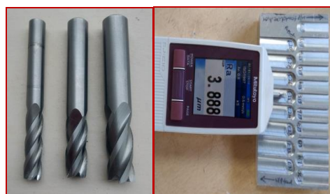
FIGURE 3.2: End mill cutters, surface roughness measuring
